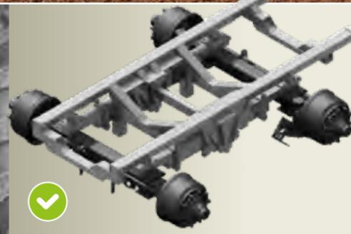
Pendelaggregat Boogie SB
