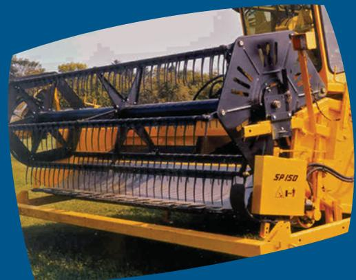
Further extend the multicrop harvesting capabilities of the 2430 by adding the SP150 cutting head for processed spinach and salad greens.
